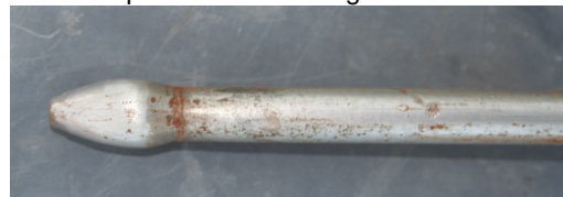
Push probe tip, the bulb aids removal from wet soil
