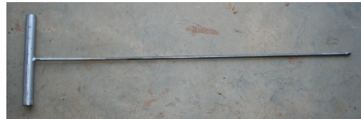
Push probe for estimating soil moisture
