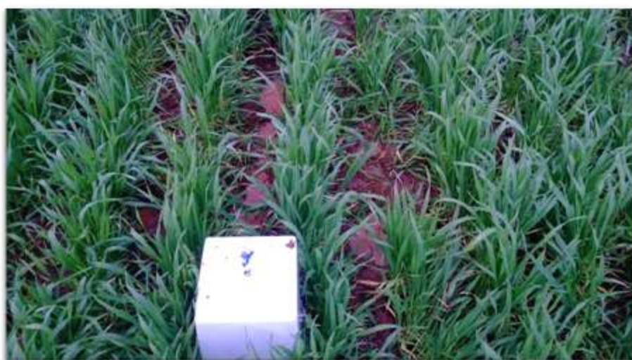
Photo: Nitrous oxide chamber in 2014 wheat crop at Hart.
