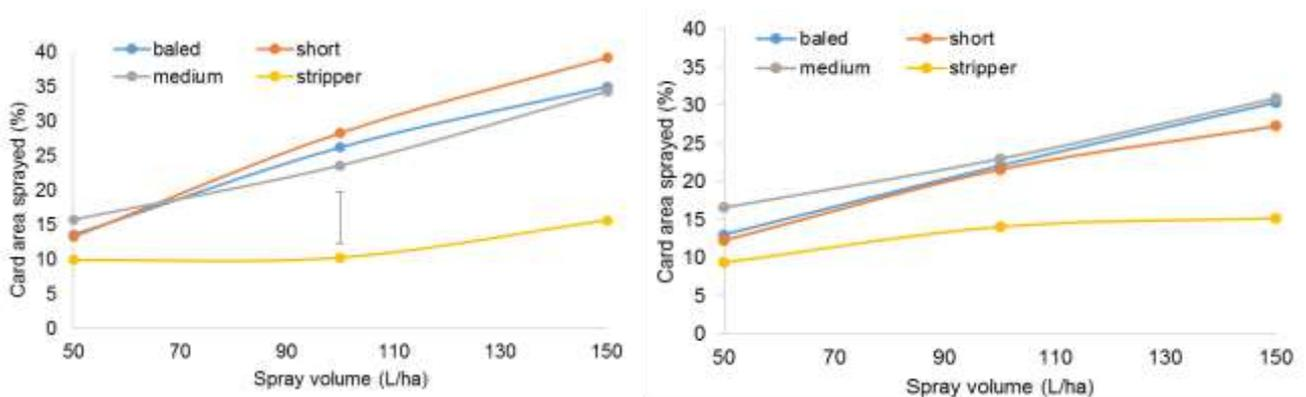
Figure 3. Area (%) of card sprayed in different stubble and spray volume combinations for medium sized droplet in 2015 (left) and 2016 (right). These are the average values for spray cards placed at the stubble base and inter-row. Signification interaction ( $P \leq 0.05$ ) for stubble and volume for both droplet sizes is indicated by the error bars.
