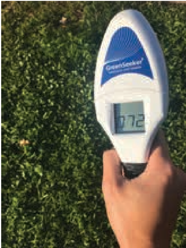
Handheld Greenseeker® for measuring assessing crop canopy reflectance in the Red and Near Infra-Red parts of the spectrum.
