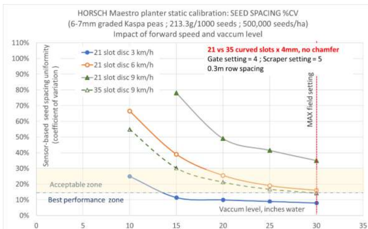
Figure 4. The impact of singulation vacuum setting and planting speed on the coefficient of variation (CV) of inter-seed spacing, with two disc plate designs.
