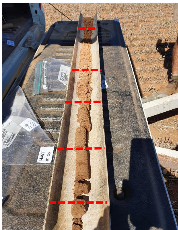
Figure 3. Conducting soil sampling to measure pre-seeding water content (%). Dashed red lines indicate breakdown of characterised soil depths at Hart.
